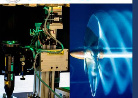
At the end of 2021, ITUKAT became operational and ranked seventh worldwide in terms of flow rate among its peers, with its large test section and a maximum achievable flow velocity of 16.5 m/s in the test section. The tunnel is powered by a 1 MW electric motor.
